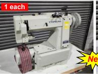
Typical M# TW4-L302U Single Needle Needle Feed Cylinder Chain Stitch
